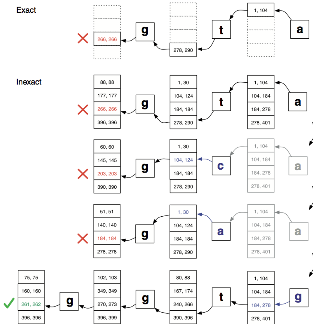
Example of inexact search of ggt a which occurs with one mismatch. (Mind the different interval definition. Here x, x denotes an empty interval.)
