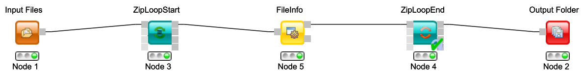
Figure 4: A minimal workflow calling FileInfo on multiple files in a loop.
