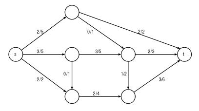
Start with the initial flow f. An edge label f/c means initial flow f and capacity c.
