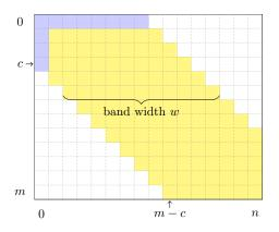
Now, we don't encode the whole DP column but the intersection of a column and the band (plus one diagonal left of the band). Thus we store only *w* vertical deltas in *VP* and *VN*. The lowest bits encode the differences between the rightmost and the left adjacent diagonal.
