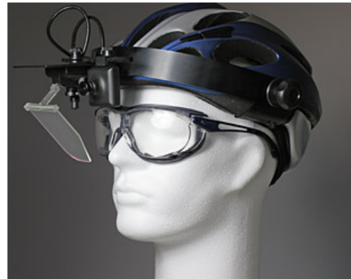
Figure 1: HED4 helmet for eye tracking
