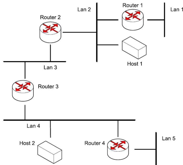
Assign IP addresses for the devices in the network depicted above. You have the IP block 137.226.0.0/16 available and should come up with a good assignment of addresses for the networks. Assume that Router 1 has an additional connection to the Internet. Based on the routing information, each router should be able to determine where all packets have to be forwarded to.
