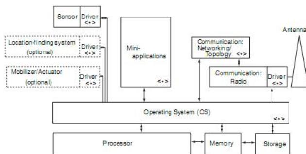
The software applications of a common sensor node, can typically be separated into five subsystems[5]:
