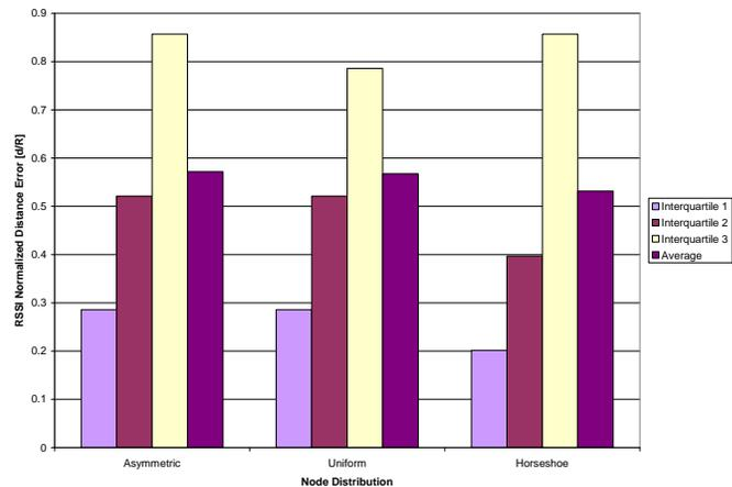
Fig. 6. Averaged normalized errors per interquartile in a asymmetrical, horseshoe and uniform distribution derived from RSSI distance estimation.
