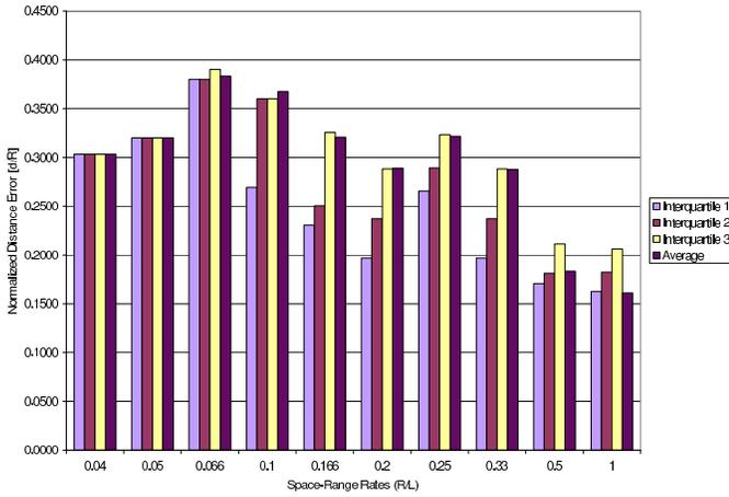
Fig. 2. Absolute normalized error in distance estimation vs. covered radio range in a simulated, uniformly distributed network .
