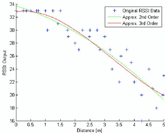
Fig. 5. Approximation of the distance between nodes based on RSSI for indoor scenario at a transmission power of 0x01.
