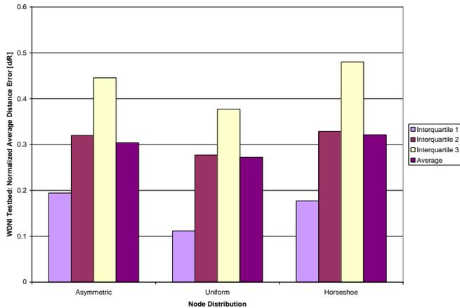
Fig. 4. Averaged normalized errors per interquartile in a asymmetrical, horseshoe and uniform distribution derived from WDNI testbed distance estimation.
