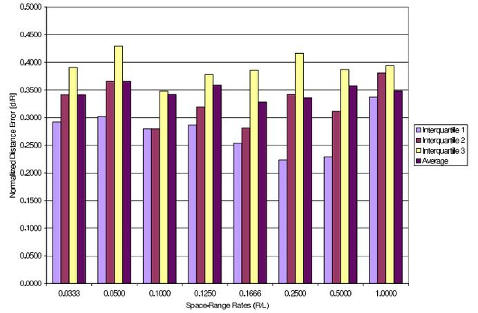
Fig. 3. Absolute normalized error in distance estimation vs. covered radio range in a simulated, near-uniformly distributed network.
