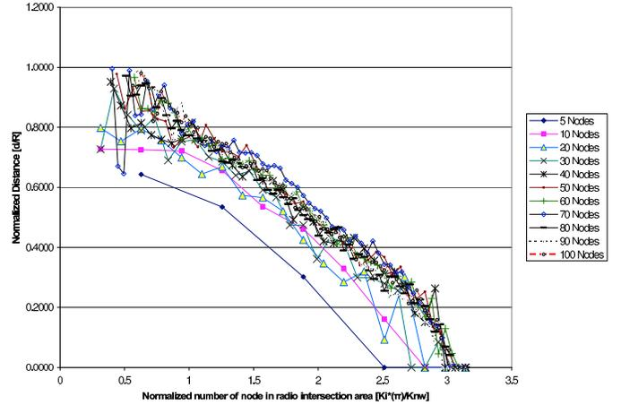
Fig. 1. Approximation graphs to estimate distance depending on  $K_i$  for different node densities.
