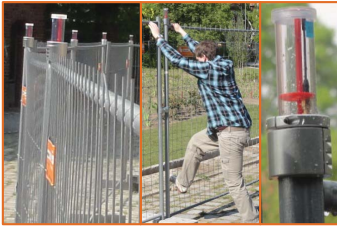
Fig. 5. Experiment at the fence & integration of sensor node into vertical fence rod
