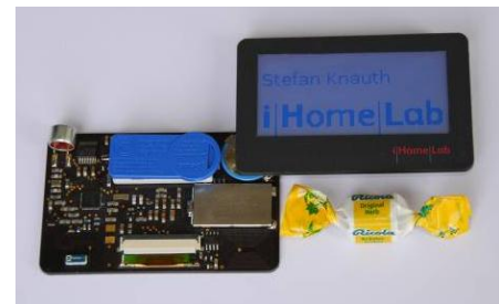
Figure 3: Name badge with transceiver, ultrasound transmitter and cholesteric LCD
