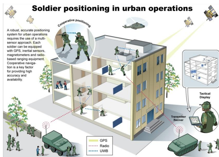
Figure 2: Illustration of cooperative positioning as an integral part of a soldier positioning system. Radio-based ranging is combined with transfer of position and error estimates, between units moving inside building as well as out to vehicle-mounted transceivers outside.
