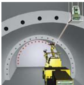
Automatic set out of drilling points and orientation of the drilling carriage
