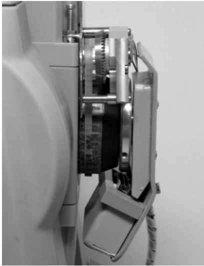
Figure 1: Modified CCD camera instead of the eye-piece. The bended small box below comprises three small electronic prints belonging to the camera. The CCD replaces the human eye and is fixed to the telescope with an identical mechanical interface as the ordinary eye-piece (ocular).
