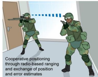
Figure 1: Illustration of opportunistic cooperative positioning between units equipped with locally-worn positioning sensors.
