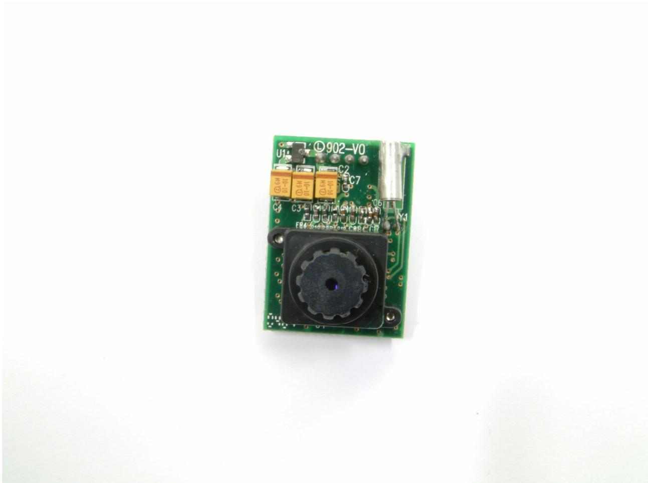
The camera module has a serial connector to connect it to the ESB.
