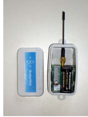
Fig. 3. Casing of a sensor node
