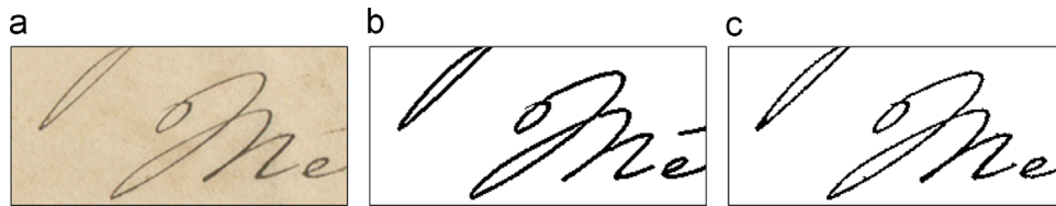
Fig. 12. (a) A sample of H06 of DIBCO 2010 is given. (b) Groundtruth. (c) Output of ROI+LogT+BR.
