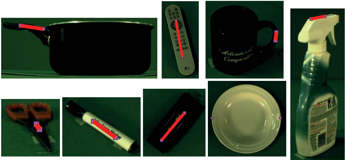
Fig. 3: Randomly sampled examples of our dataset with grasp annotations. Grasp region attribute is defined by two end points (magenta patches in the figures). We take convex hull of the two points as valid grasp region except for the bowl category.
