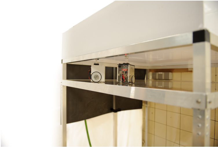
Fig. 3. The wheeled robots are moving on a transparent plastic plate in a space below the water tank. A camera on the floor is used to track the individual robots that each have three infrared LEDs inset in their baseplate.
