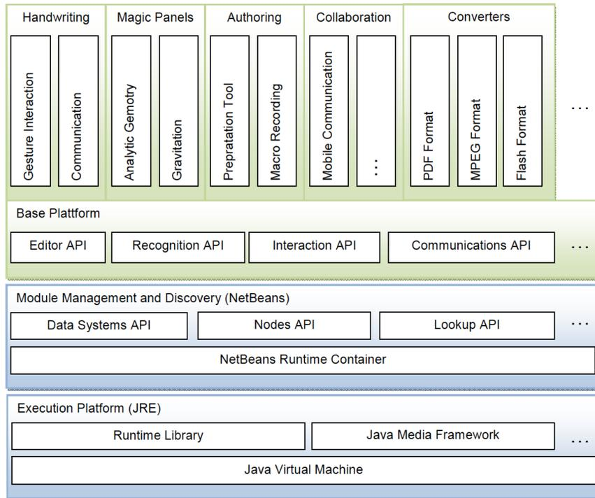
**Fig. 1.1** Modular structure of PowerChalk
