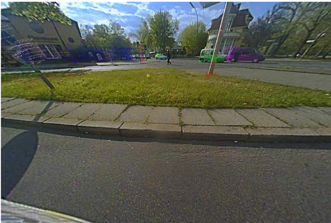
Figure 4: Example for the projection of LiDAR data onto a camera image. The different colors refer to different objects found by a clustering algorithm.
