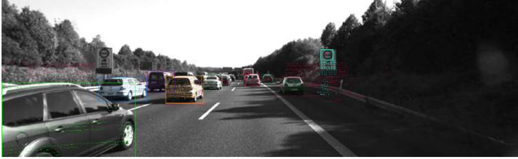
Figure 42: Sensor Fusion evaluation on the image 000111.png of sequence 20 of the KITTI dataset. Only objects that could be mapped to a LiDAR object are shown. The colors are the same for a bounding box and the corresponding LiDAR object.
