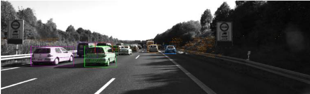
Figure 43: Sensor Fusion evaluation on the image 000129.png of sequence 20 of the KITTI dataset. Only objects that could be mapped to a LiDAR object are shown. The colors are the same for a bounding box and the corresponding LiDAR object.
