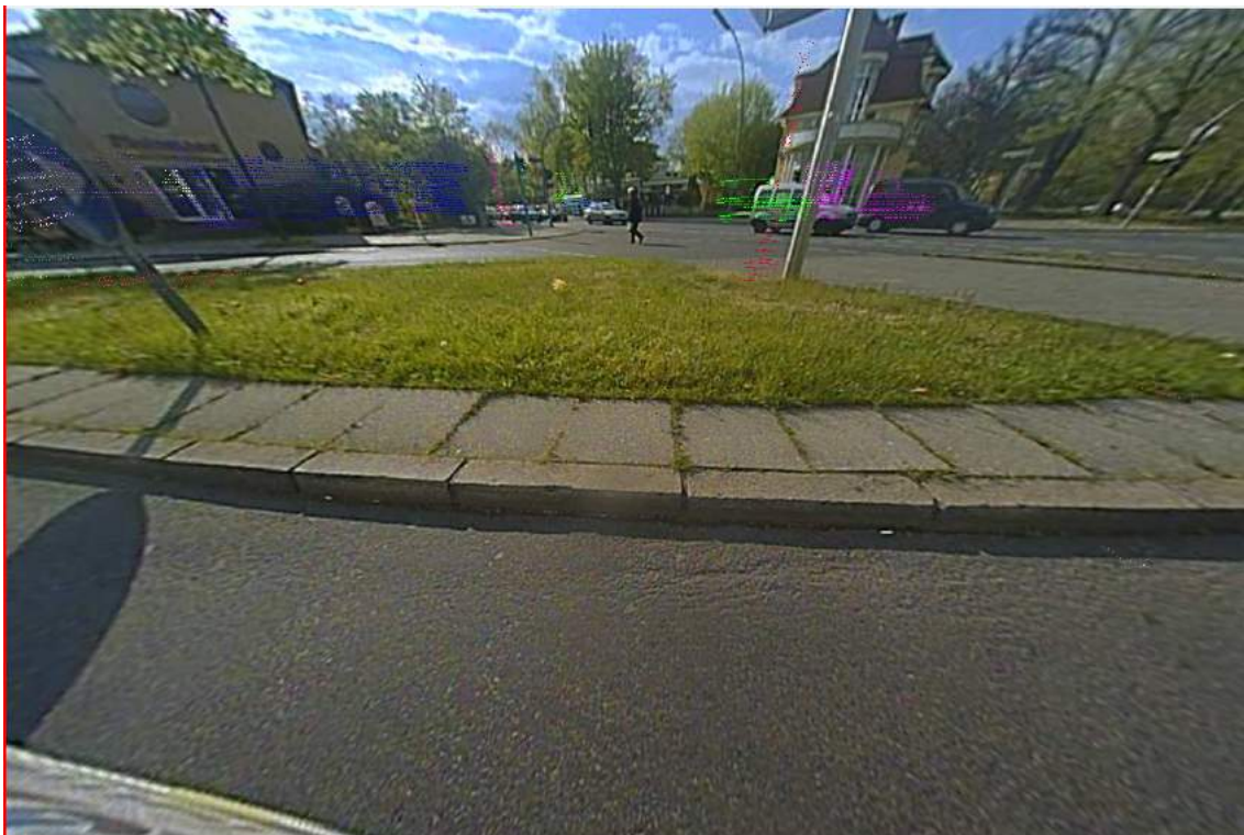
Figure 39: Poor calibration of the LiDAR to the left camera..
