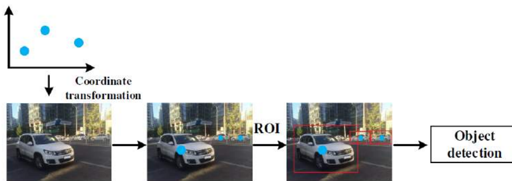
Figure 5: Illustration of the working principle of Data Level Fusion [27].
