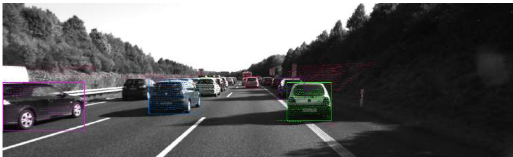
Figure 41: Sensor Fusion evaluation on the image 000000.png of sequence 20 of the KITTI dataset. Only objects that could be mapped to a LiDAR object are shown. The colors are the same for a bounding box and the corresponding LiDAR object.
