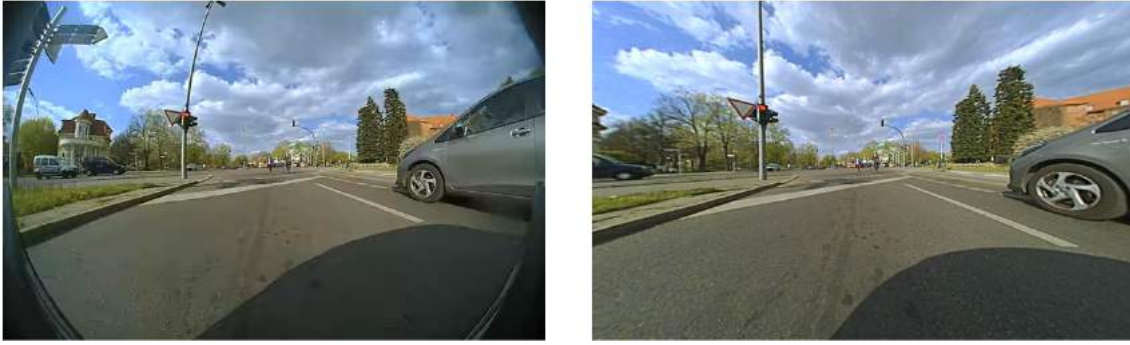
Figure 15: Rectification results based on an example image. Note the imperfection of the rectification process: (left) Distorted image taken with a camera, equipped with a fisheye lens. (right) Same image, but after rectification.
