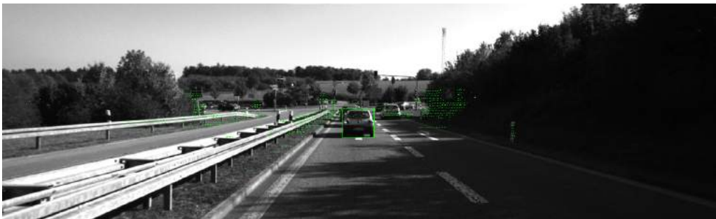
Figure 44: Sensor Fusion evaluation on the image 000753.png of sequence 20 of the KITTI dataset. Only objects that could be mapped to a LiDAR object are shown. The colors are the same for a bounding box and the corresponding LiDAR object.
