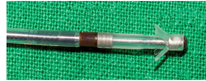
Figure 1.7: Picture of the distal end of a lead [howtopace.com/basics-of-pacing-leads]
