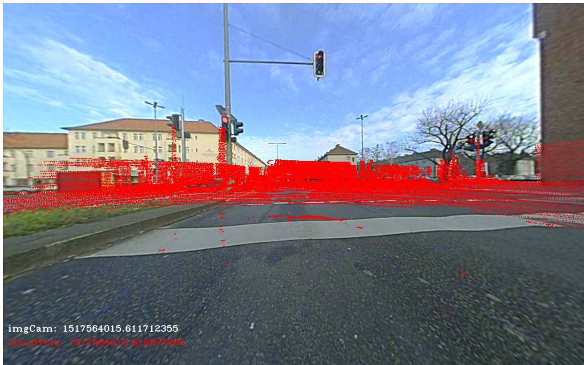
Figure 4.15: MIG SatCam RGB Color Image With Point Cloud Overlay
