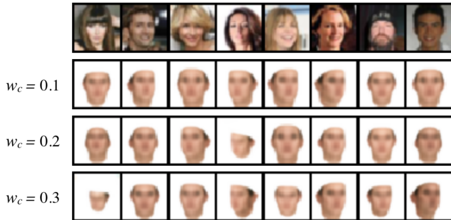
Figure 4.14: Influence of w_c on the predictor - Higher values of w_c are decreasing the capability of the predictor to predict correct label vectors for real images.
