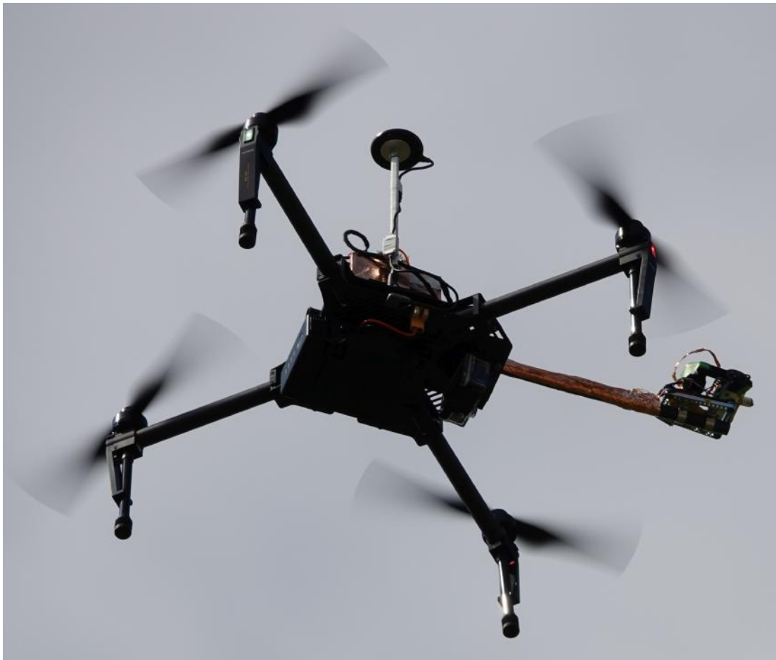
Figure 28: The Neurocopter in air doing extracellular recordings of a honeybee
