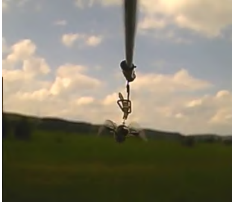
Figure 30: A honeybee attached to the Neurocopter showing flight behavior during a forward flight. The rolling shutter effect lets the bees wings look curved.
