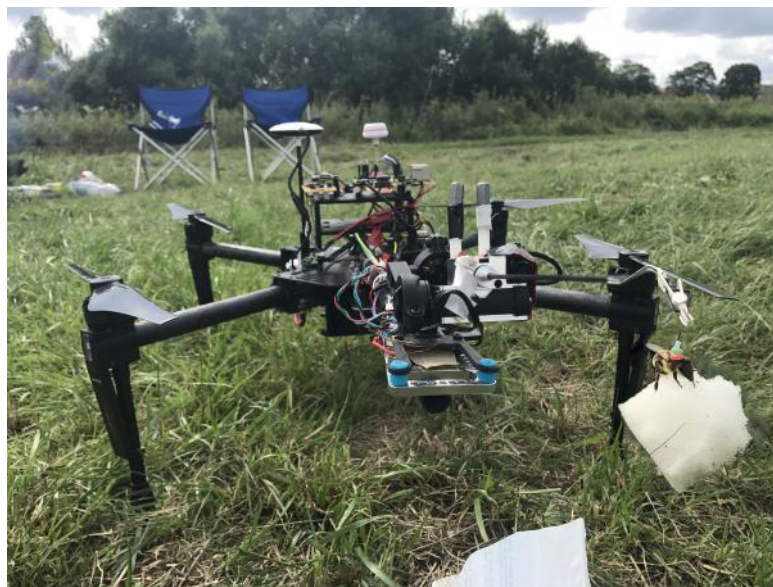
Figure 29: A bee attached to the Neurocopter in Amöneburg (Hesse)
