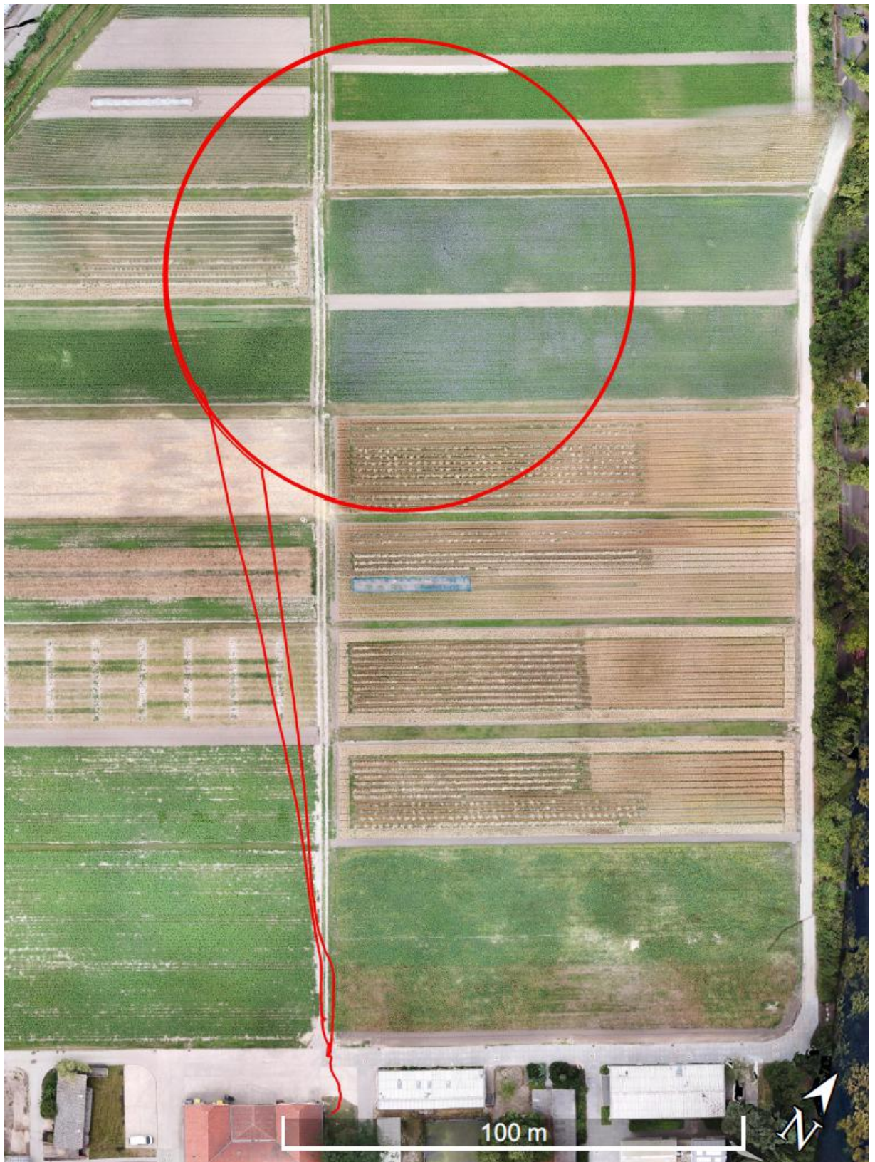
Figure 43: Circle pattern flown on the 05.07.2018 at the Julius Kühn-Institut. The radius of the circle is 50m, the altitude 19 m and the speed was 23 km/h. The way to and from the automatically flown circle is also plotted. For more information about that experiment read section 7.1.1. The background map was created by the author with a drone (for the mapping process see section B.1 in the appendix).
