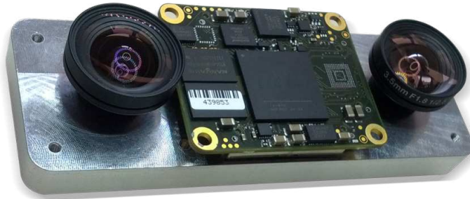
FIGURE 1.1: An example of a stereo camera used by the Autonomos GmbH.
