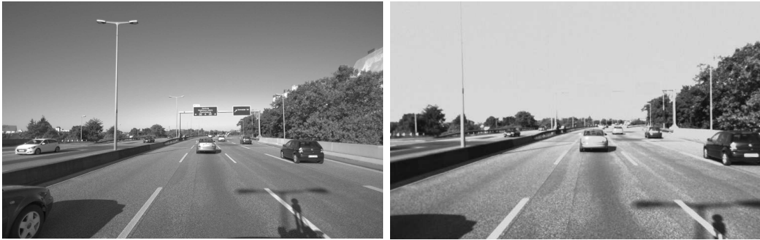
FIGURE 6.4: Comparison of the details of the stereo image (right) and the monocular image (left). Consider the center of the images, the left image of the monocular camera reveals a traffic sign that is not visible on the right image of the stereo camera.
