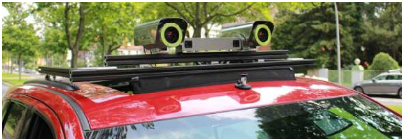
FIGURE 5.1: A monochrome stereo camera system (in the center) and two monocular color cameras (on the sides) are used for experiments in this work, mounted on a vehicle roof and aligned to the driving direction. Only data from the stereo camera was used for the evaluation.
