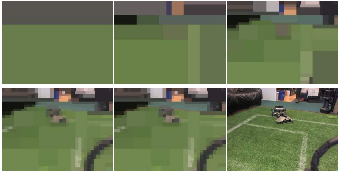
Figure 4.2: Processing steps of the field contour extraction; nodes are displayed in their mean color. Top left: PLANT after first split. The split matches the field contour roughly. Top center: Increased number of nodes. Corner of the field becomes visible. Top right: Increased number of nodes. This segmentation would be sufficient at this point. Bottom left: Final PLANT. The algorithm stops at a certain threshold. Bottom center: Superimposed resulting field contour as a red line. Bottom right: Original image including the field contour.
