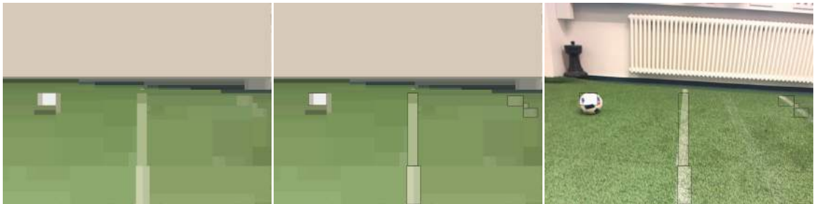
Figure 4.4: White blobs for ball detection. Left: Illustration of PLANT that is built to find white blobs. Center: Black rectangles mark white blobs. Right: Marked white blobs in the original image.
