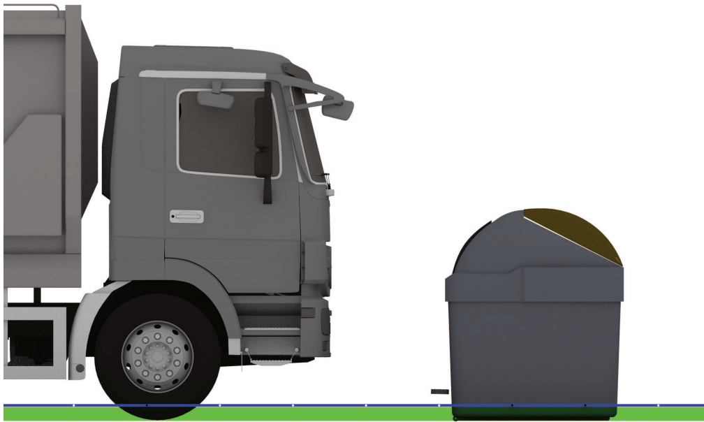
Figure 4.2: A threshold plane (blue) separates points that are retained (green) from points that are discarded.
