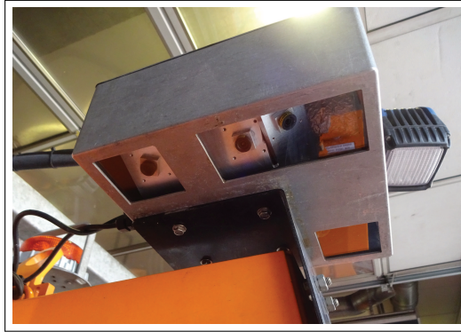
Figure 3.4: A two stereo camera system used by the Autonomos GmbH and for experiments in this thesis[19]. There are two such rigs mounted at the rear of the truck.
