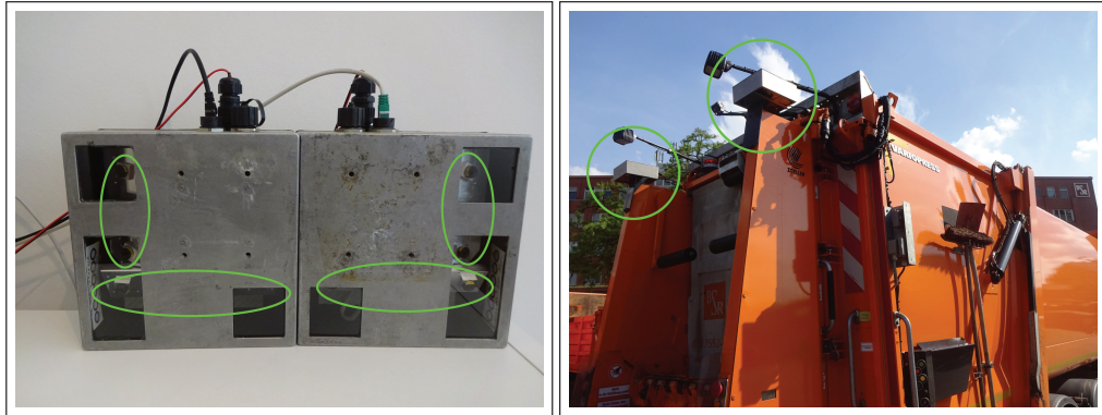
(a) The used camera rigs. The green ellipses mark the stereo cameras. (b) Garbage truck with the mounted camera rigs (green circles).
