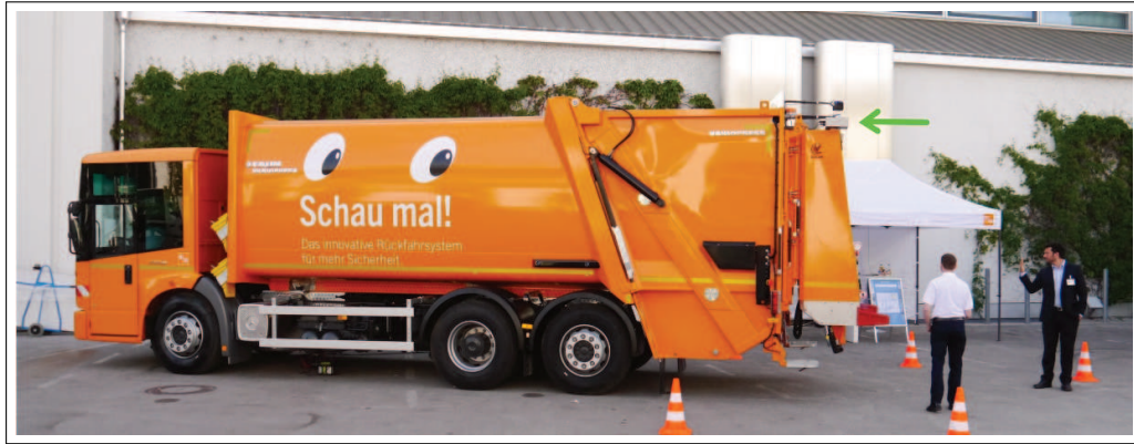
Figure 1.1: A truck from the RAS project with a stereo camera rig on the upper rear.
