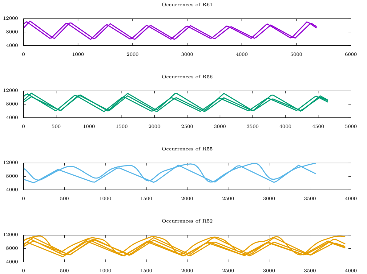
FIGURE B.1: This plot shows all occurrences of the rule set S_1 . This set contains four rules. Each rule's occurrences are plotted into a single panel. The x-axis contains the uptime in milliseconds. The y-axis corresponds to the angle of Myon's left shoulder.
