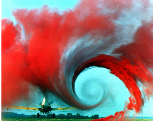
(b) Wingtip vortex forming in the wake of an aircraft. Author: NASA.
