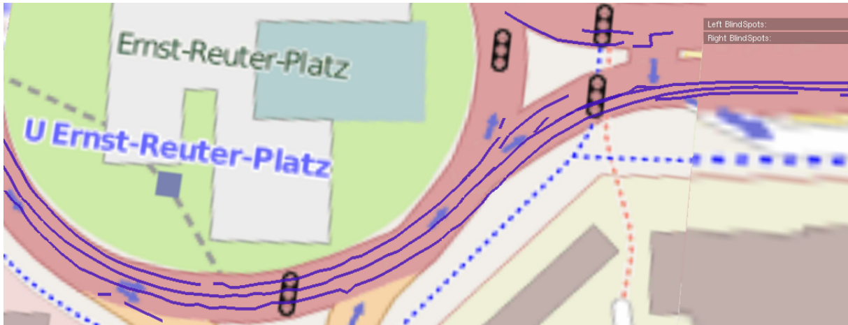
Figure 5.3: "Clusters" generated from the tracked swarm data using the described adaptation of the "Extracting representatives of GPS points" method from [GLJ10]
