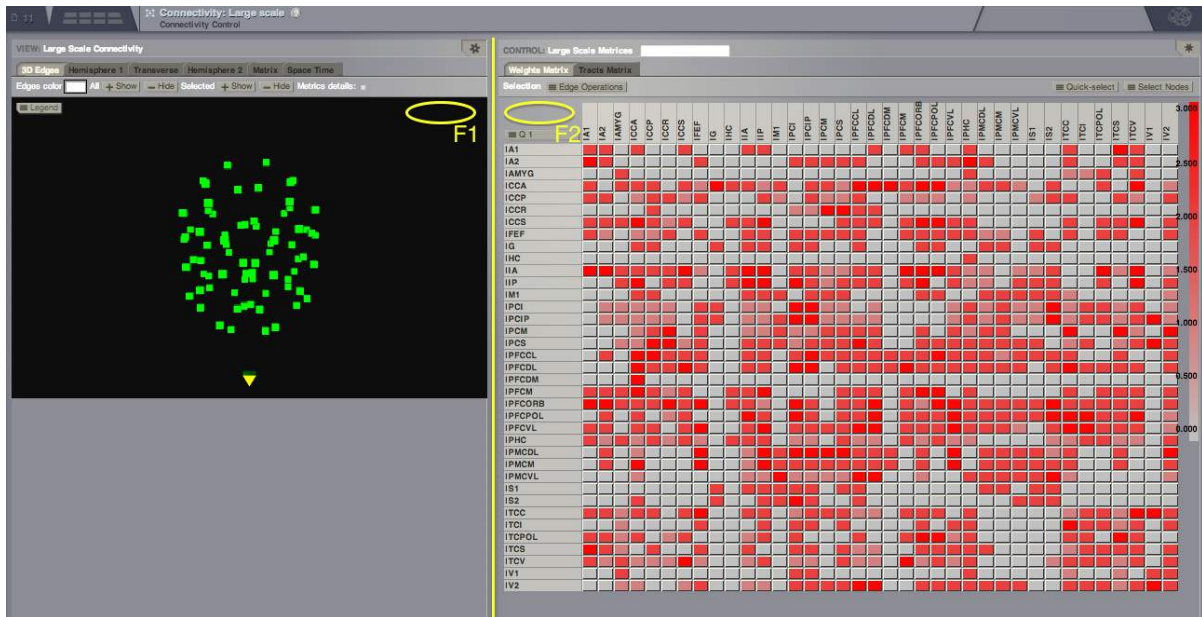
Figure 1.6: Screen splitting - The Connectivity Interface arranges the main area into two frames: the Viewer (F1) and a Control panel (F2).
