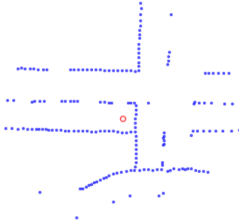
Figure 4.2: The resulting set of points used as B for tracking, where the red circle marks the center of mass. The robot's front points right.
