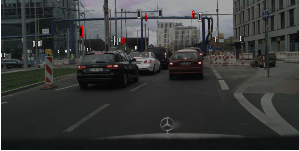
Figure 4: Example image from the training set of the DTLT dataset with labels
