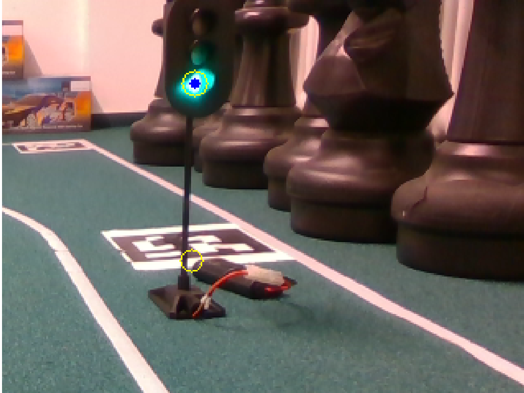
Figure 4: Points where color was tested marked in yellow and the detected traffic light marked in blue
