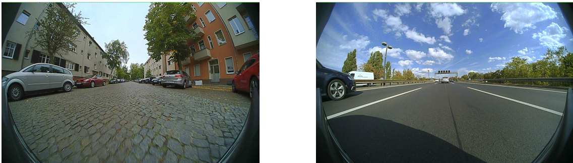
Figure 4.2: Example images from the dataset, in which either the road boundaries are very unclear because of parking cars and missing lane markings (left) or in which the roads are very well-maintained with clear lane markings as seen on highways (right).
