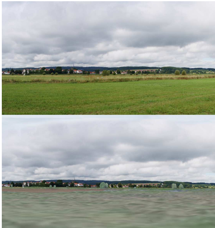
Illustration 3.7: To validate the alignment of the skydome, the sections of the 2D panorama (upper images) are compared with renderings of the 3D model (lower images) from the same viewpoint from which the panorama had been taken (viewpoint 1). The images show that the objects (such as bushes) are approximately at the same position and similar in size.
