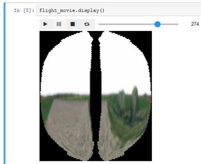
Illustration 6.1: The Radar Track module is meant to be used interactively with Jupyter Notebook (IPython). This image is a screenshot of the IPython Widget that is used for displaying the flight movies. The widget provides a slider and play/pause functionality, so one can simply browse through the frames in the FlightMovie.
