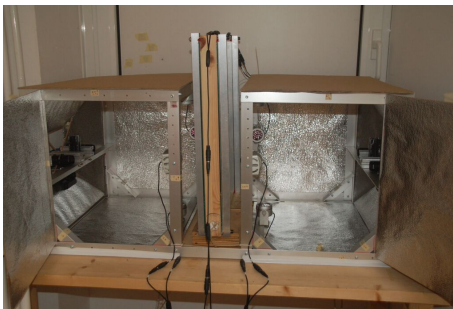
(a) The hardware setup consisting of a comb, located inside an aluminum scaffold that is equipped with cameras and infrared LED lamps.
