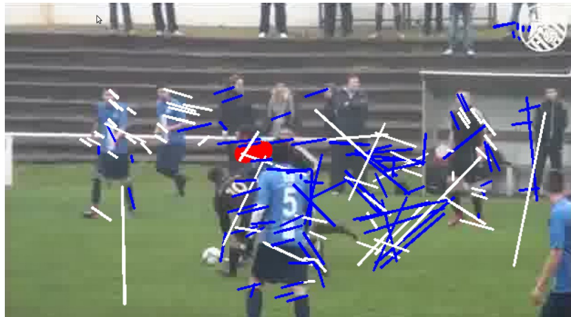
Figure 5.6: Before filtering out outliers with the unbiased estimator. White lines – all tracked features, the blue ones – outliers.
