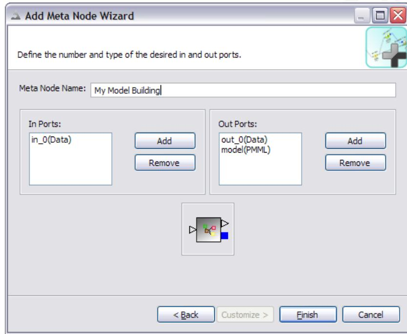
On this page you can add or remove in- and out-ports of the template. An icon at the bottom immediately gives you a preview of the node. When you add a port to the template you can choose the type for the port:
