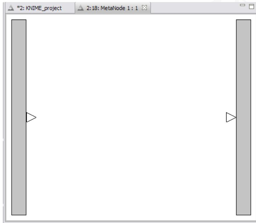
The in- or out-ports are fixed to the so-called workflow port bars, which can be moved and resized. The data connected to the in-port from outside appears inside the meta node editor in the in-port. And vice versa: the data connected to the inner out-port appears in the outer out-port.
