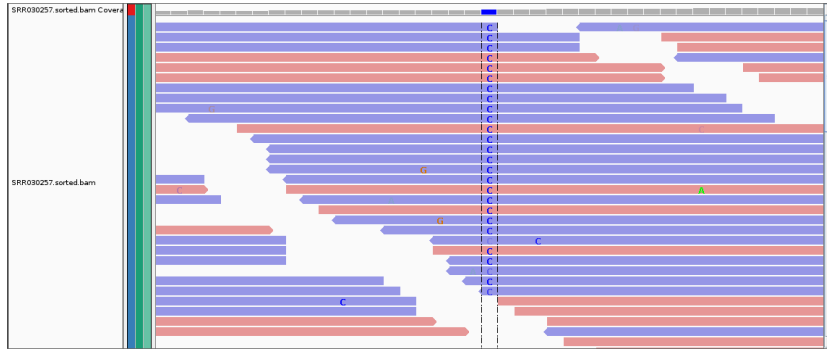
Figure 2: Visualization of mutation at position 555154, ref=A, alt=C, DP4=0,0,7,17. This means there were no reads supporting the reference sequence, but there were 7 forward reads (red) and 17 reverse reads (blue) supporting the ALT call.
