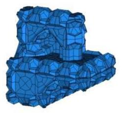
version of Boy's surface, one produces a regular subdivision for a "pile of cubes" that has a subdivision of the Boy surface as a dual manifold. The result (file C4P\_Boy\_C3B\_with\_dual\_Boy\_surface.hexas) is then lifted to a 4-polytope by a prism-type construction. (See [3] for details.)
