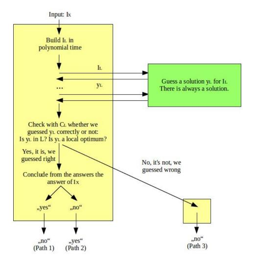
Figure 2: Nondeterministic Turing Machine that verifies that X is in co-NP
