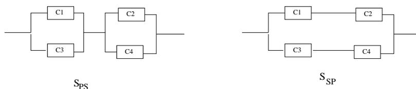
Figure 1: Series of parallels and parallel series components
