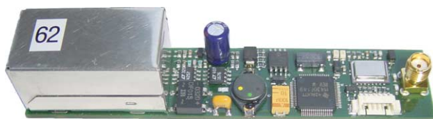
Fig. 7. Embedded Web Server (EWS) connecting the sensor network with Ethernet.
