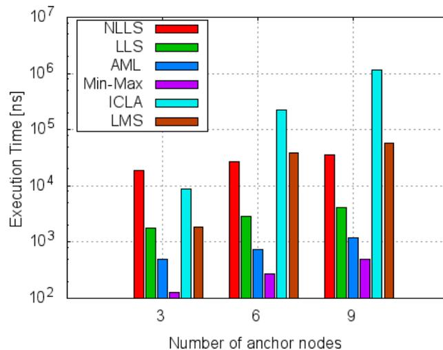
**Fig. 9:** Execution times of the six localization algorithms
