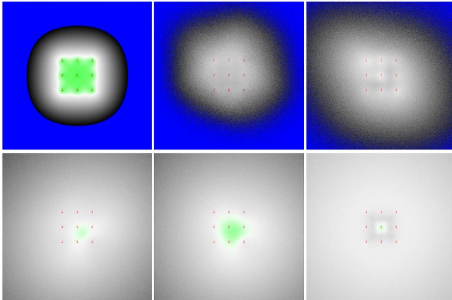
**Fig. 10:** The average spatial error distribution of the six simulated algorithms (1000 simulation runs). The algorithms are from left to right: Min-Max (480% average position error compared to expected distance error), ICLA (408%), AML (340%), LMS (202%), LLS (188%) and NLLS (138%).
