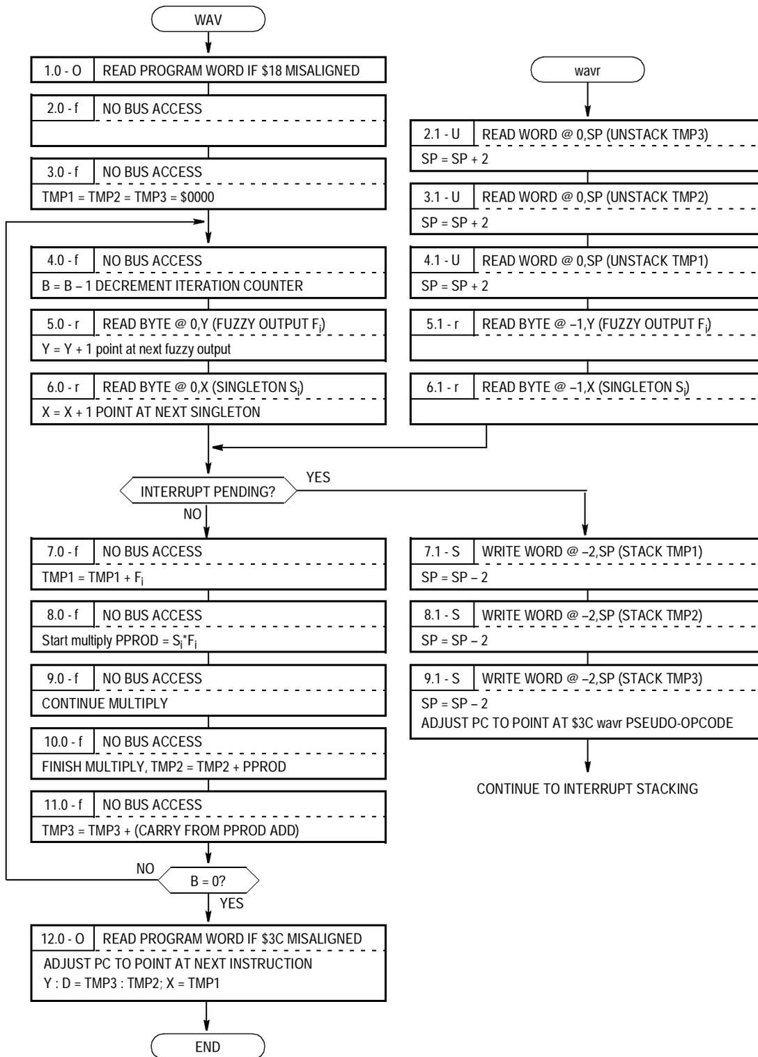
**Figure 9-11. WAV and wavr Instruction Flow Diagram**
