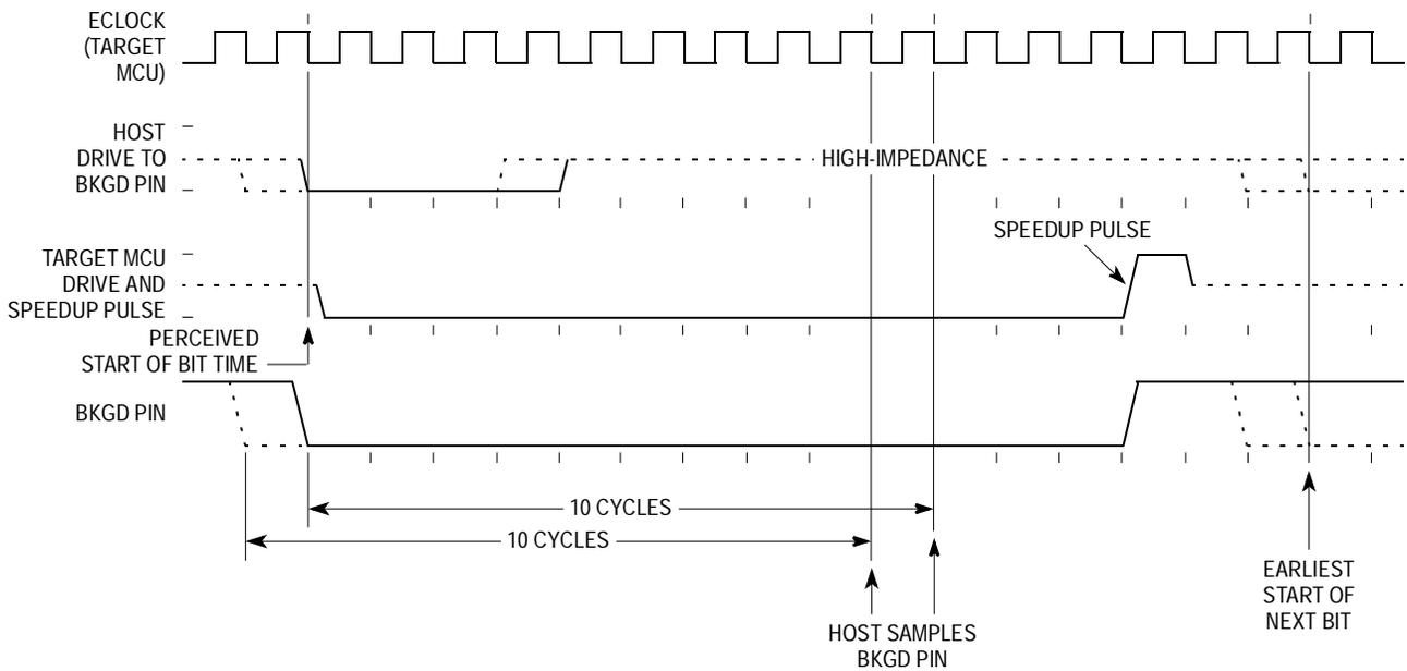
**Figure 8-4. BDM Target to Host Serial Bit Timing (Logic 0)**
