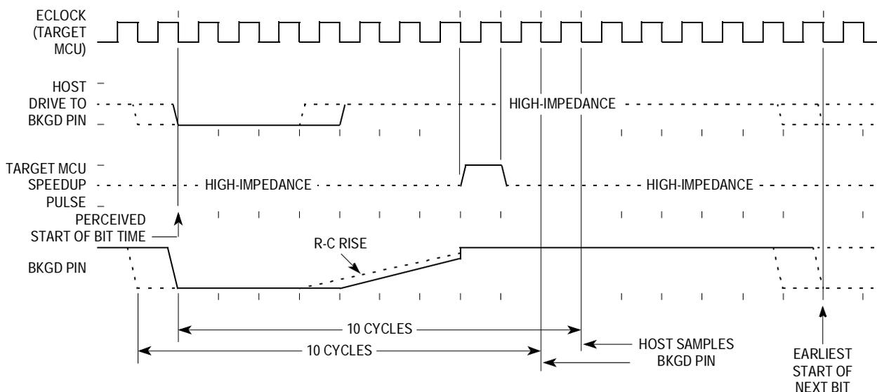
**Figure 8-3. BDM Target to Host Serial Bit Timing (Logic 1)**
