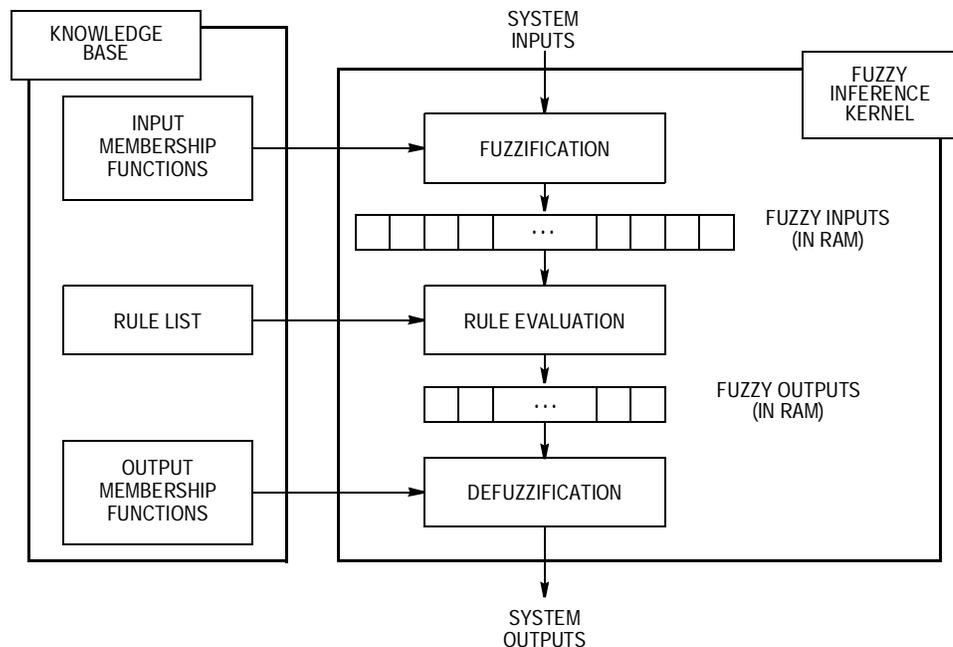
**Figure 9-1. Block Diagram of a Fuzzy Logic System**
