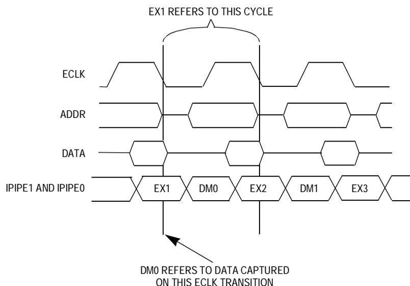
Figure 8-1. Queue Status Signal Timing
