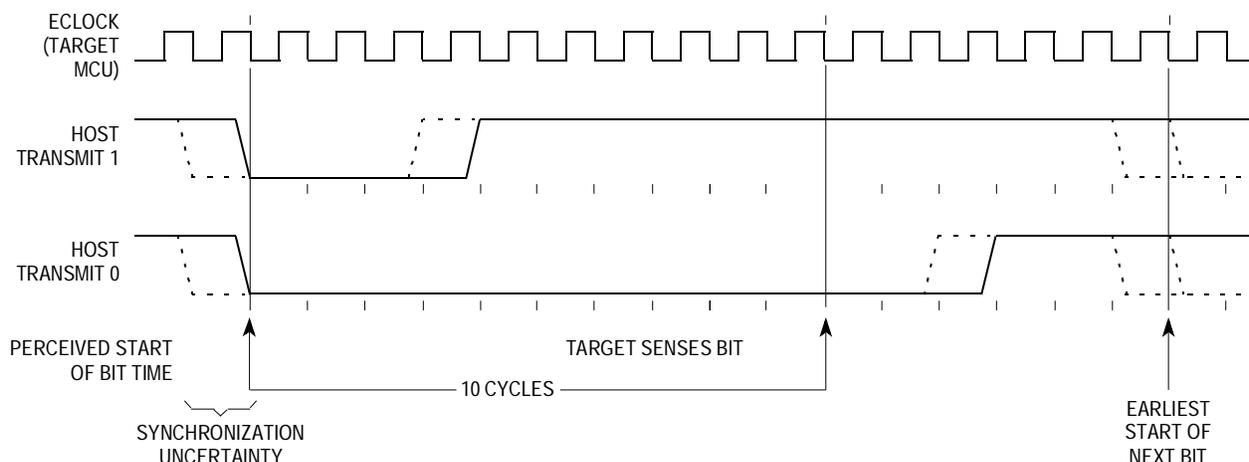
**Figure 8-2. BDM Host to Target Serial Bit Timing**
