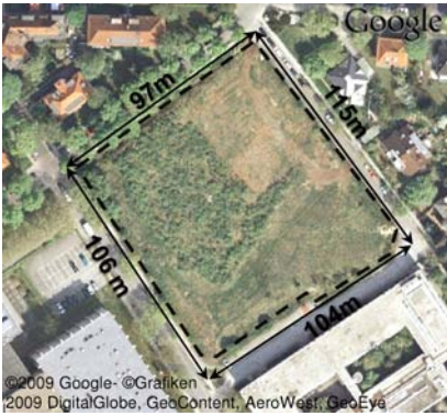
Figure 7: Construction Site with Highlighted Run of Construction Fence
