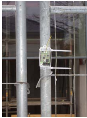
Figure 8: ScatterWeb MSB Sensor Node Attached to a Construction Fence
