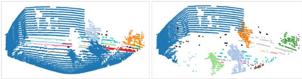
Figure 3.16: Example of point cloud clustering without and with preliminary ground segmentation.
