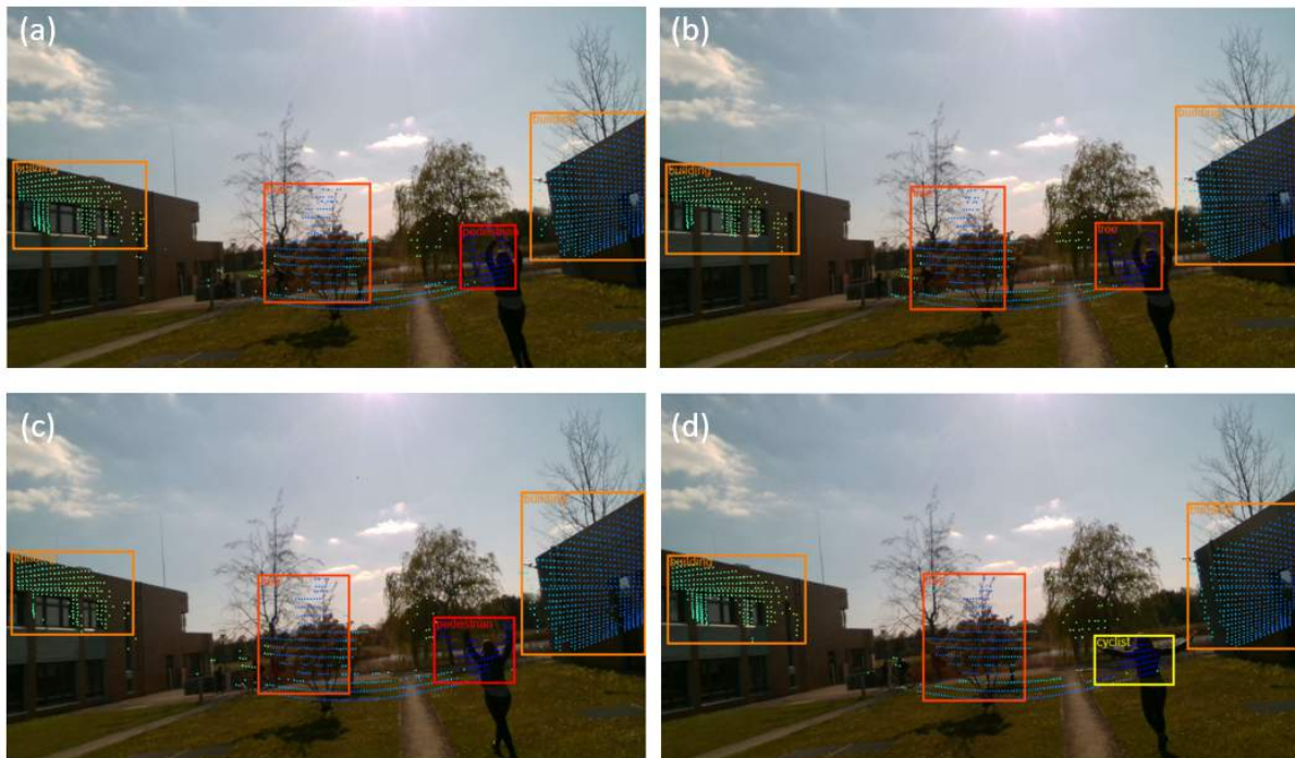
Figure 4.31: Classification of the person based on position of hands (pedestrian, tree, cyclist)
