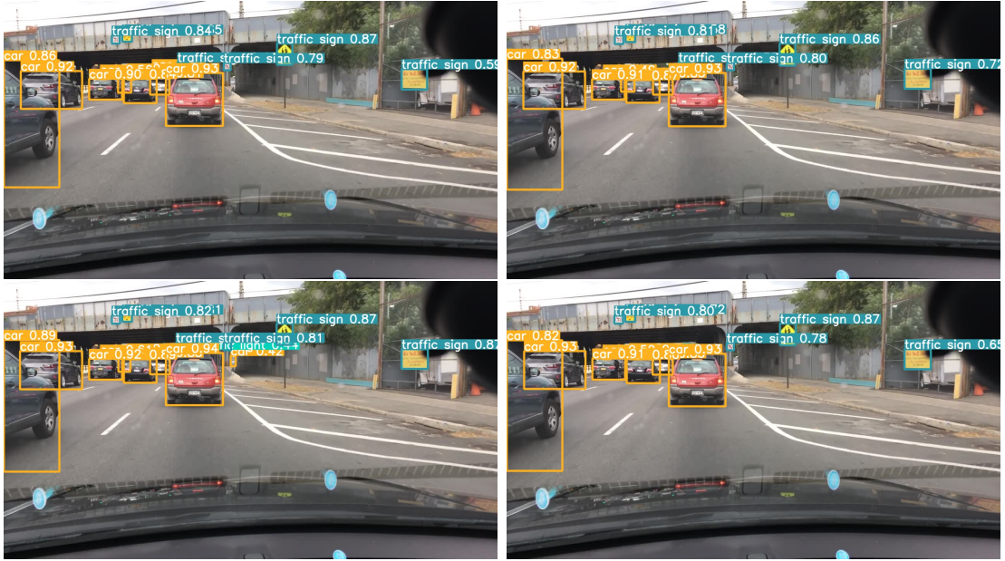
Figure 29: Example detections for models trained with four different sampling strategies. Top left: Model trained with random sampled data. Top right: Model trained with LP-based stratified data. Bottom left: Model trained with LP-based stratified data with maximized instances. Bottom right: Model trained with iterative stratified data.
