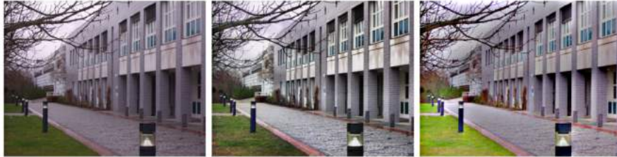
Figure 1.1: Example for a differently enhanced image Left: raw image Middle: CLAHE enhanced image Right: MSRCR enhanced image (raw image from [12])
