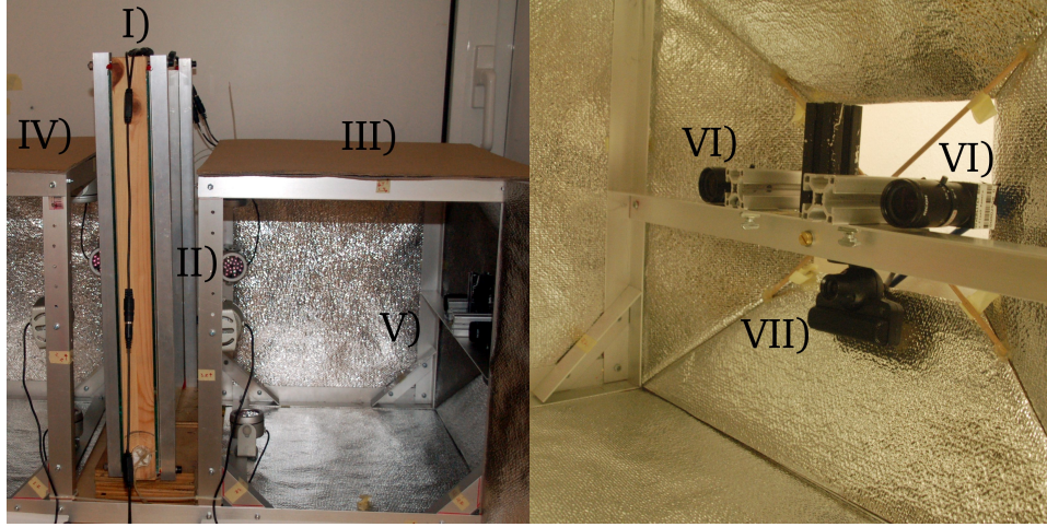
Figure 4.6: Beesbook experiment site setup. Marked items are: I) observed honey bee comb, II) one red light device, III) right side of observation cage, IV) mirrored left side of observation cage, V) right side camera array, VI) high resolution cameras, VII) PlayStation Eye Camera.
