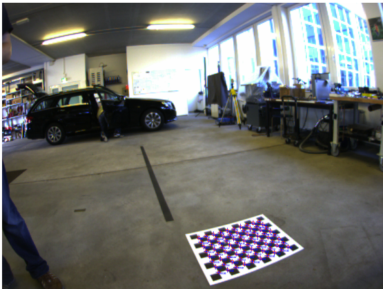
(a) Camera view of the pattern aligned with the car.
