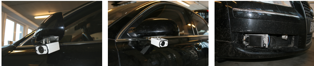
(a) Camera with housing mounted to mirror (b) Camera with housing mounted to mirror (c) Side radar sensor mounted to bumper
