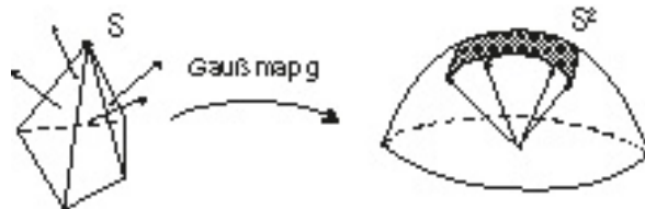
FIGURE 7.1. The Gauß map assigns to each point p \in S of a surface its normal vector n(p) \in \mathbb{S}^2 . At edges and vertices of a polyhedral surface the image of the Gauß map is the spherical convex hull of the normal vectors of adjacent faces.
